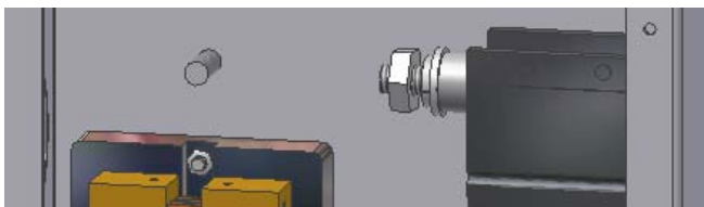
5/16" stud for battery negative tie point
