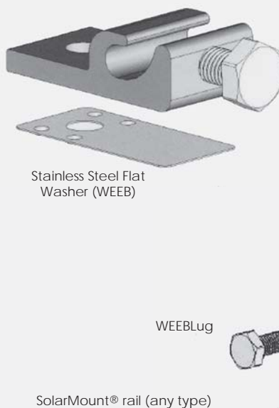
Figure 2. Insert a bolt in the aluminum rail or through the clearance hole in the stainless steel flat washer. Place the stainless steel flat washer on the bolt, oriented so the dimples will contact the aluminum rail. Place the lug portion on the bolt and stainless steel flat washer. Install stainless steel flat washer, lock washer and nut. Tighten the nut until the dimples are completely embedded into the rail and lug. The embedded dimples make a gas-tight mechanical connection and ensure good electrical connection between the aluminum rail and the lug through the WEEB.
